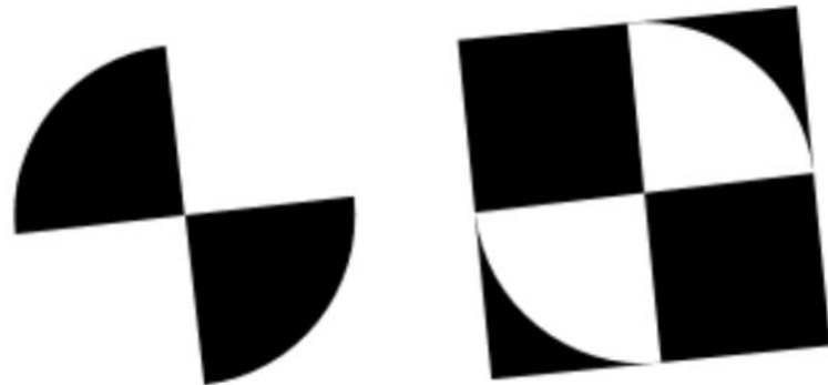
Fig. 2: Slanted edge reticle
