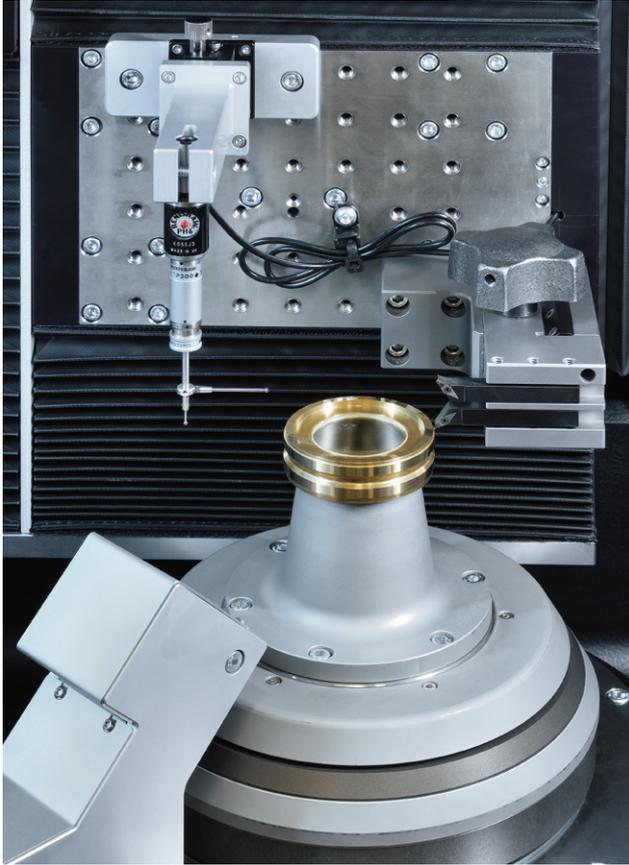
The automatic adjustment chuck aligns the optical axis of the workpiece precisely with the rotation axis of the turning station. After a tactile measurement of the flange surfaces and the external cell diameter, machining begins.
