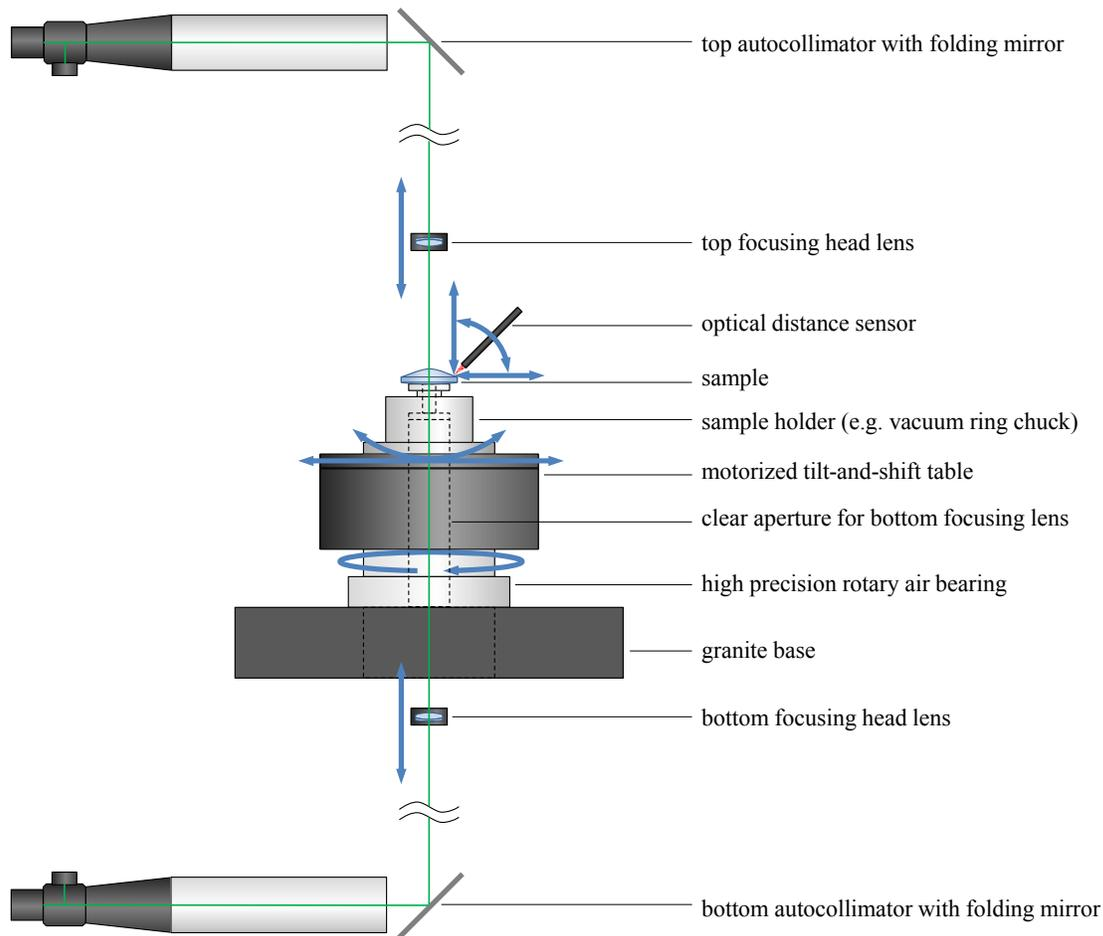
Figure 3: components of the AspheroCheck UP system
