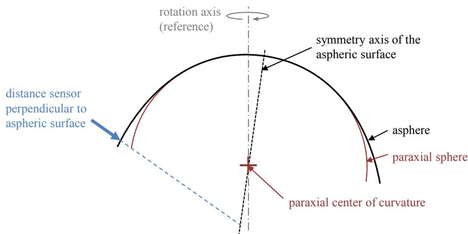
Figure 2: aspheric surface tilt measurement using a distance sensor
