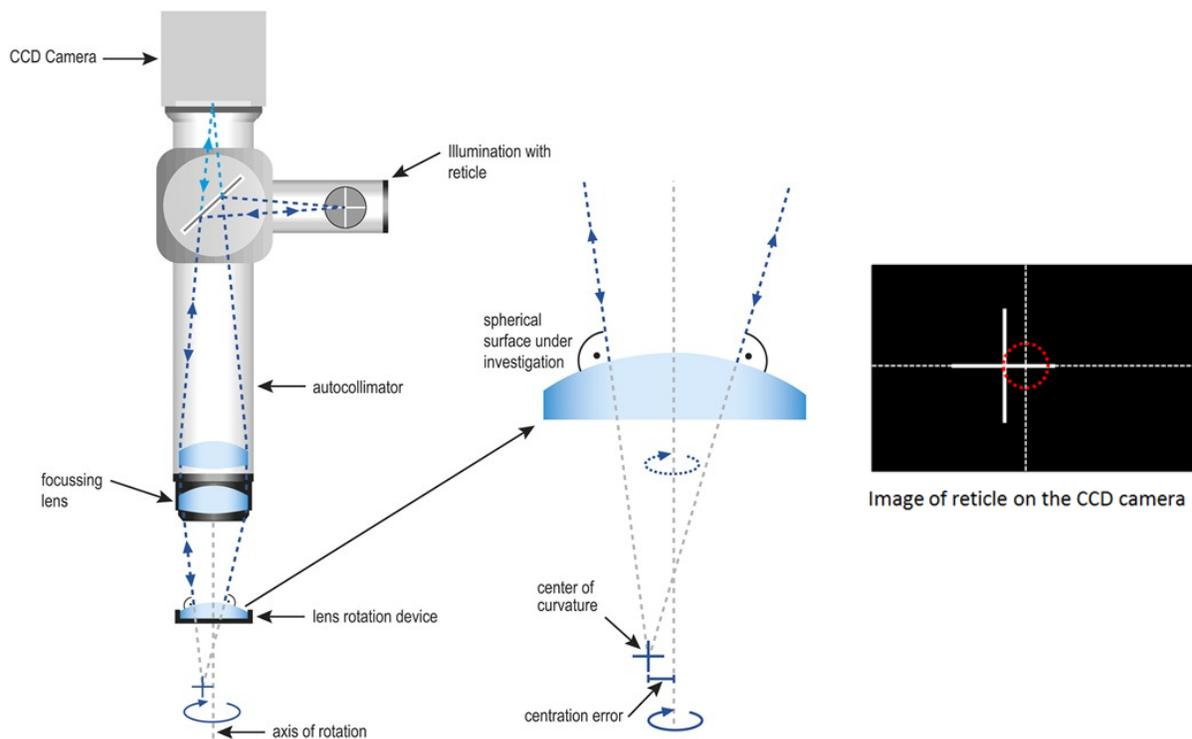
Figure 1: Measurement of the centration error in reflection mode with autocollimator and reticle
