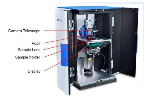
The Trioptics ImageMaster Lab VR system can be used to evaluate the effectiveness of Fresnel lenses in VR headsets.
