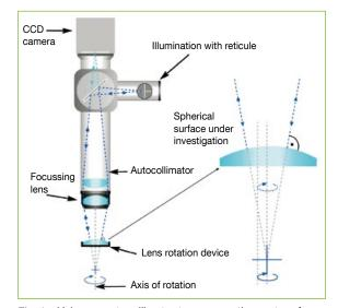
Fig. 1 Using an autocollimator to measure the center of curvature of a lens.
