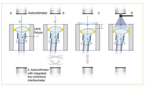
Fig. 6 a) The adhesive is applied to the edge of the lens and the spatial positions of the lens axis and cell axis are measured; b) The lens is aligned in the cell in four degrees of freedom; c) The axial gap between the apex point of the lens and a reference surface is measured and the lens adjusted axially; d) The adhesive is cured.
