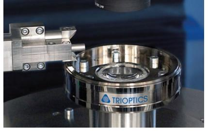
Mounted lens aligned, machined and tested with an alignement turning machine from Trioptics.
