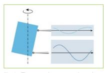
Fig. 2 The measuring sensors determine the shift and angle of inclination of the cell.
