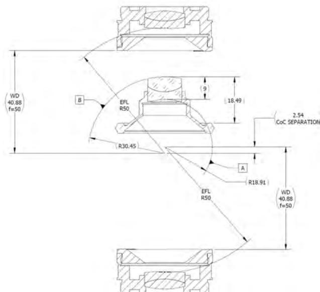
Figure 7 - Illustration of problematic case where the center of curvature of two different optical surfaces are nearly coincident (within less than 3 mm)
