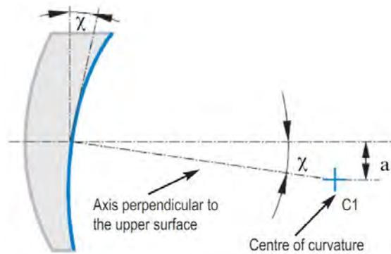
Figure 4 - Schematic diagram of the surface tilt error
