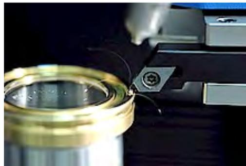
**Figure 3 - ATS 200 machining a mounted lens**
