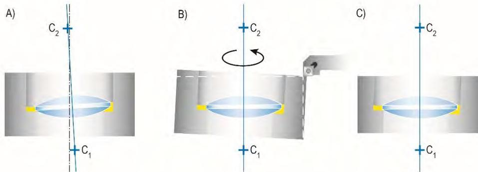
**Figure 2 - The alignment process: A) optical axis C1-C2 is determined; C) cell is tilted and decentered so optical axis C1-C2 is coaxial with the mechanical spindle axis, and then the outer cell surfaces are machined; B) after machining the outer cell surfaces run true with the optical and mechanical axes**
