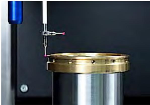
Figure 6 - The integrated gauges of the ATS 200 measure the diameter of the mounted lens
