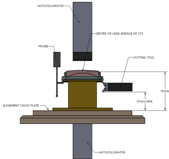
Figure 8 - Illustration of typical workpiece setup showing geometric design constraints
