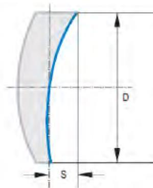
Figure 5 - Surface tilt error given as eccentricity
