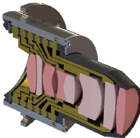
Figure 11 - Jenoptik Microscope for Display Inspection
