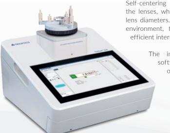
Self-centering mechanical chucks are used to hold the lenses, which can be easily adjusted to various lens diameters. Optimized for use in the production environment, the entire device is equipped with efficient internal vibration damping.
